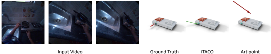
Fig. 8: Example results for articulation estimation. Red arrows refer to revolute joints and green arrows refer to prismatic joints. In the left example, iTACO predicts incorrect joint types, whereas Artipoint is correct. However, both methods struggle with small parts such as the stove knob shown here.
